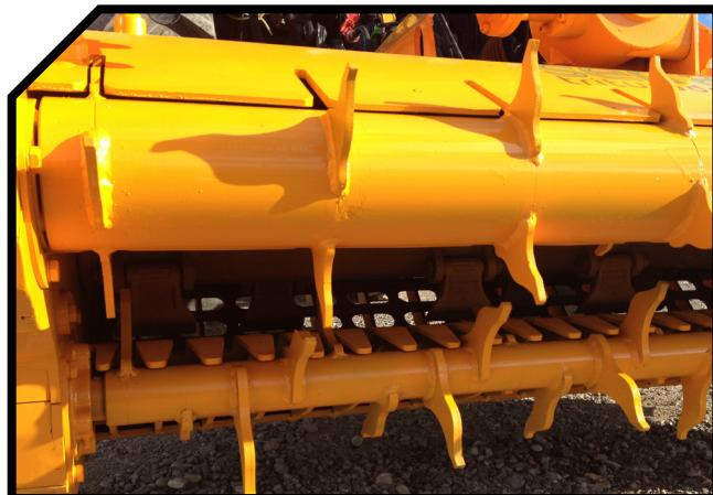
**Criba trasera dentada recambiable**
